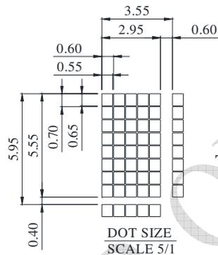
The non-specified tolerance of dimension is ±0.3mm.
